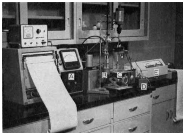
Figure 1 —Instrumental setup for the automated determination of dissolution rates. Key: A, pH-stat titrator; B, titration buret; C, dissolution test apparatus; D, peristaltic pump; and E, spectrophotometer.
